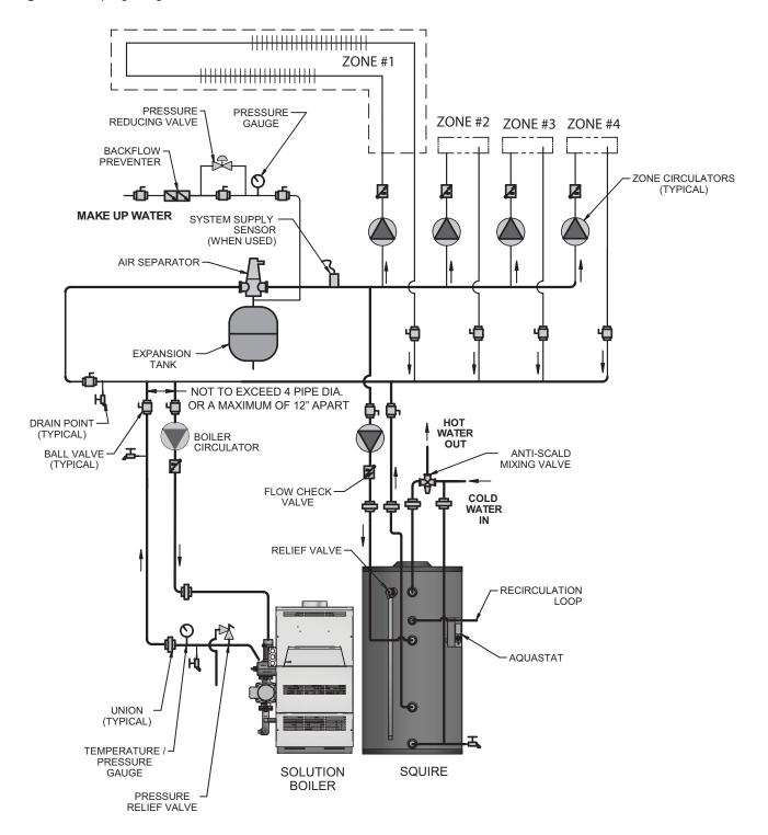
Figure 3-2 Piping Diagram Zoned with Valves
